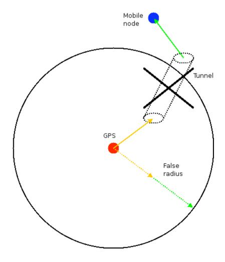
Because we can't allow tunneling to "spoof" a short distance (by forming a "wormhole" between two TV white space based sub-meshes), the distance information must be conveyed at the MAC layer. The white space devices must enforce the rule that distance information cannot be tunneled, so there's no way to "spoof" a short distance. This must be enforced by the hardware and drivers in the white space devices.
