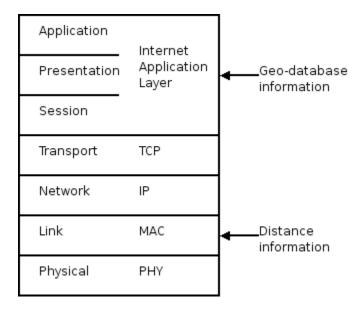
The geo-database will provide permissions as a function of distance from the known, geolocated node. This will be combined with distance information to calculate the permissions for each mobile node. Access to the geo-database is best left to a layers above TCP/IP. This allows maximum flexibility (bridging, routing and tunneling). Since it doesn't matter at all what path this information takes, there's no reason to do anything else.
