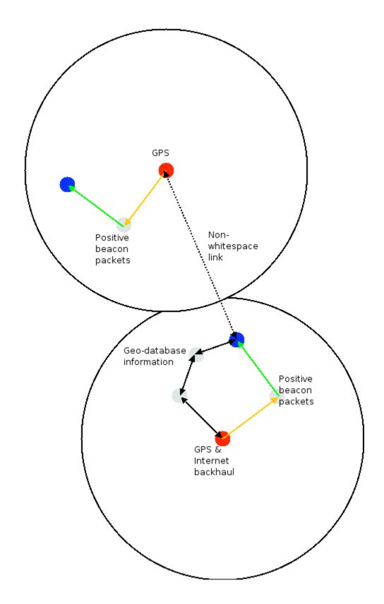
Even in a heterogeneous mesh network (using TV white space as well as other RF links), it is still the case that only one node in the overall mesh needs access (by whatever
