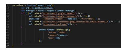
**Figure 2.** Javascript module of Kimsuky's "SHARPEXT" Chrome extension malware, which specifically searches for SSO-authenticated email account access. (Image: Volexity<sup>4</sup>)
