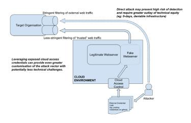
**Figure 1.** Accessing the legitimate infrastructure's underlying cloud hosting environment provides greater opportunities for attack tailoring.
