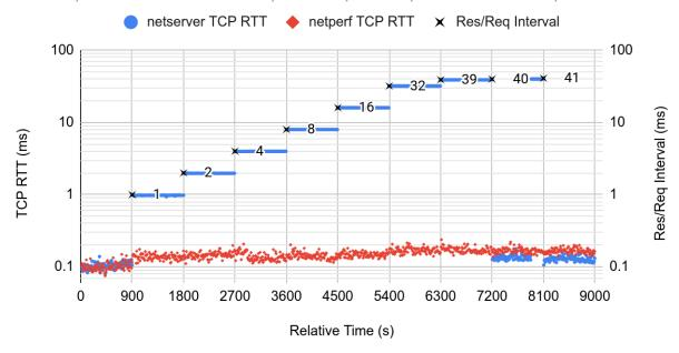
What we see here are the TCP-measured RTTs for both sides of the connection(s) - netperf and netserver. When the netserver side application receives a complete request it will immediately send a response, so the ACK of the request will be piggybacked with the response without any additional delay. This then is why the TCP RTT on the netperf side is as low as it is.
