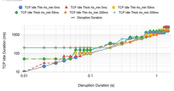
The logarithmic axes may be a bit unpleasant but are necessary at this level since we are spanning a few orders of magnitude along both axes. Basically what this shows is that for Disruption Durations less than the value of rto\_min, the TCP connection will go idle for the length of rto\_min.
