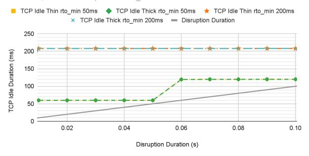
The sharp-eyed will notice that for the 50ms value of rto\_min, our idle duration isn't actually 50 milliseconds, but closer to 60. While we configured the rto\_min in units of milliseconds, those got converted to something else in the Linux kernel 6.5 networking stack, and the granularity of that conversion makes the timeout greater than 50 milliseconds. A similar effect can be seen with the 200ms value of rto\_min.
