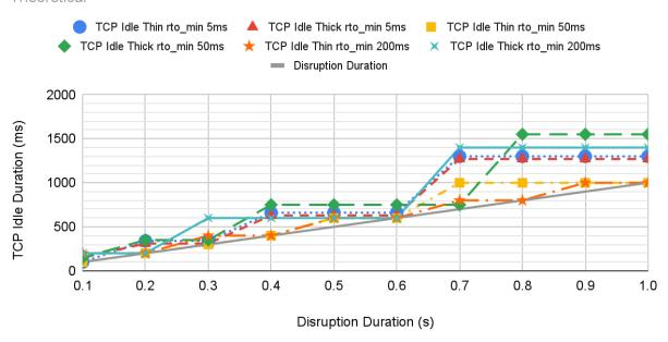
Without getting into too much detail, we can see how "thin" continues until it hits its limit before starting doubling. And we can see that sometimes, the TCP Idle Duration can be longer for a smaller value of rto\_min when the timeouts are "thick." The smaller rto\_min has been able to double more often and can "leapfrog" the longer rto\_min. But the longer rto\_min will then itself leapfrog.
