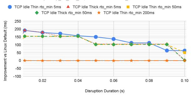
The "5ms thin" line rather nicely shows how net.ipv4.tcp\_thin\_linear\_timouts works with the improvement changing by ~5ms or so at a time until the doubling-range is reached. Now on to the middle "region" of Disruption Duration:
