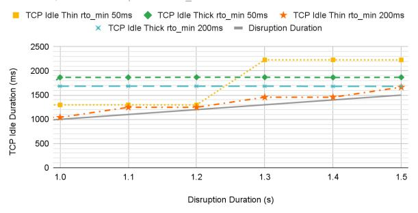
We no longer double again as we get to a backout duration of 1.5 seconds. And so why this chart's y-axis tops-out lower than the same chart from <a href="Theory">Theory</a>. It isn't always in our favor though. In the theoretical chart for rto\_min of 50 milliseconds and "thin" retransmissions we went only as high as 1800 milliseconds but here we end up between 2000 and 2300 milliseconds.
