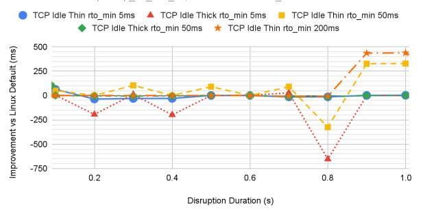
We start to see some "convergence" of the different values. A reminder about the paucity of datapoints hiding the stair-stepping of reality. We can see that for 5 ms "rto\_min" there are a few regions where we will have TCP idle a little longer than it would have with the default ("thick" retransmissions and an "rto\_min" of 200 milliseconds).
