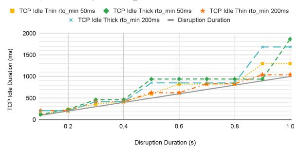
In the Theoretical chart for this region of Disruption Duration, TCP Idle Thick (200ms) was up to only 1400 milliseconds. But since the underlying starting point was more like 209 milliseconds, our doubling has taken us to not quite 1700 milliseconds. Similar things have happened with rto\_min of 50 milliseconds. Which is why, when we look at the last region of Disruption Duration:
