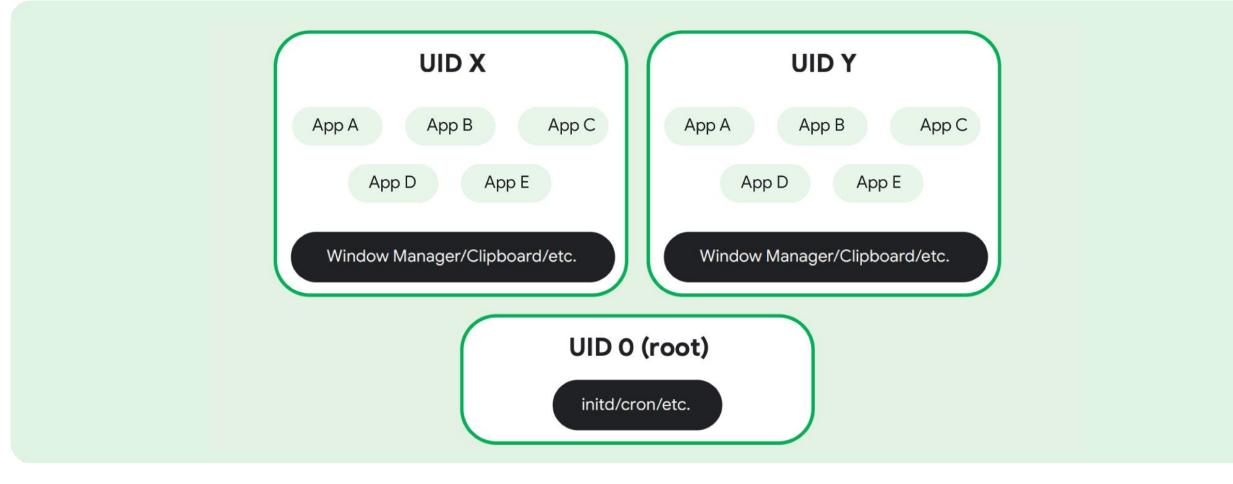
Figure 1. Relationship between users, apps, and system services in Linux.
