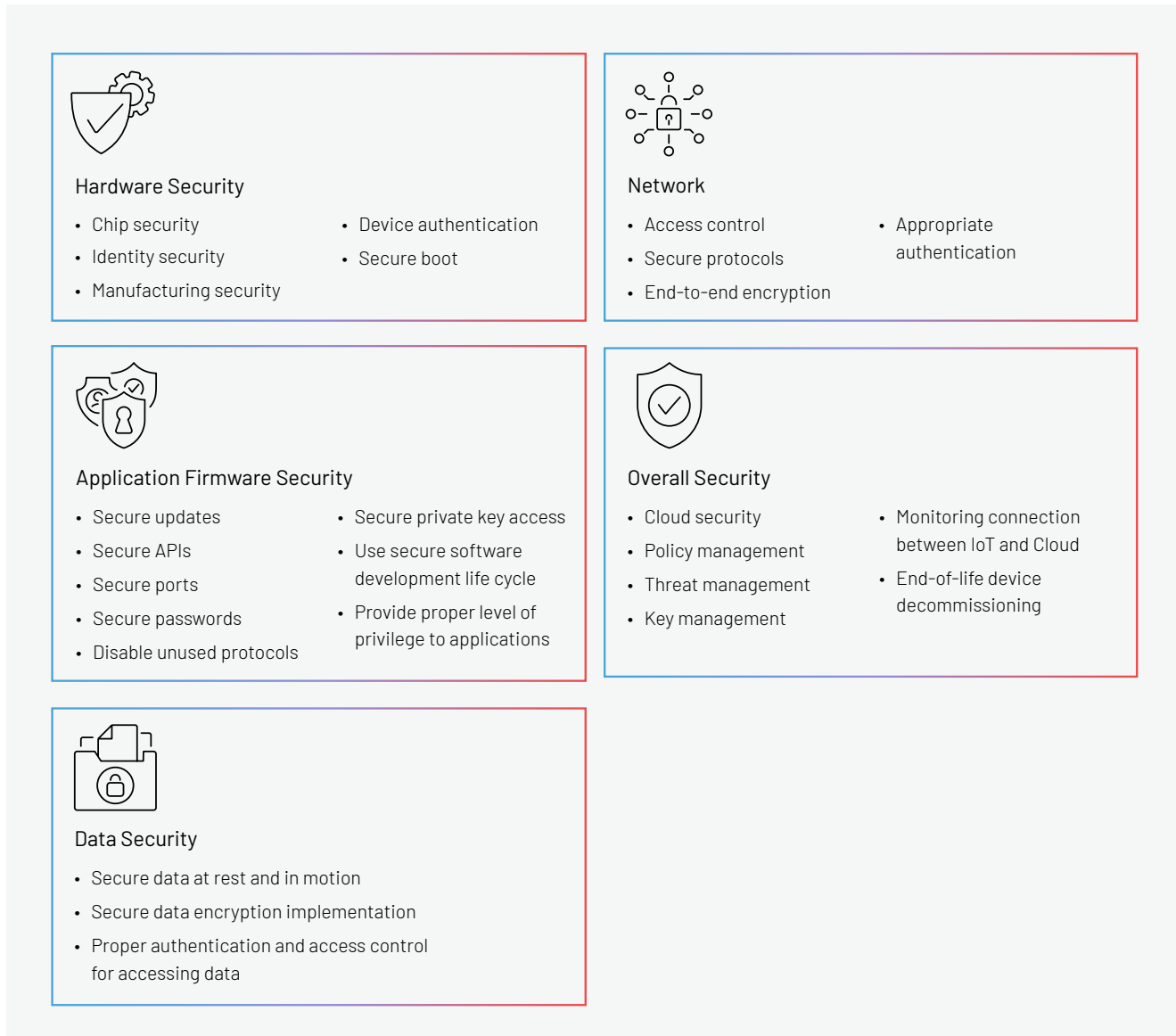
FIGURE 3: Considerations for securing IoT devices
