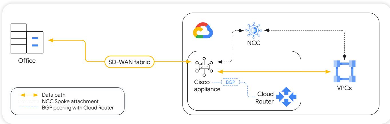
Cisco Cloud OnRamp automation for this step provides peering-based connectivity intent management in the user interface and APIs.
