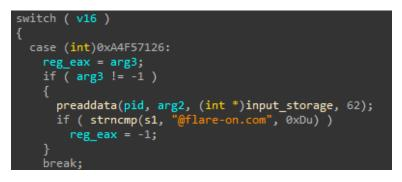
Figure 25: Watchdog handler that checks if the flag meets the flag format
