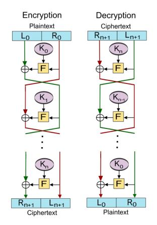
Figure 21: Diagram of a Feistel Cipher (from https://en.wikipedia.org/wiki/Feistel\_cipher#/media/File:Feistel\_cipher\_diagram\_en.svg)
