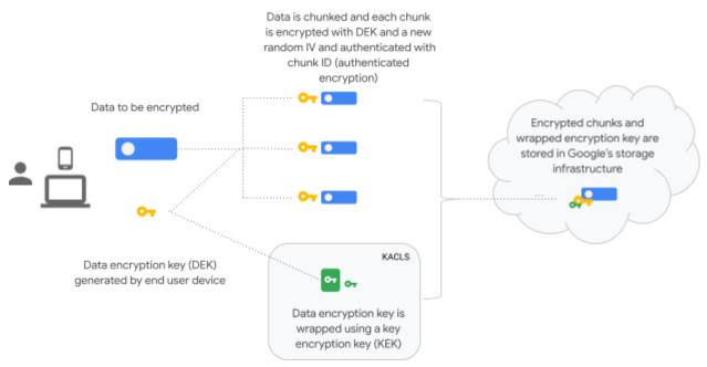
Data Encryption using Google Workspace Client-side encryption
