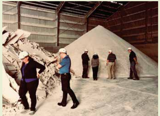
Google, Building Product Ecosystems, and contractors tour the PABCO Newark facility site to explore opportunities for drywall recycling at Charleston East and Bay View. The project teams collected all gypsum wallboard scrap on-site and returned it to the facility to be manufactured into new drywall.
