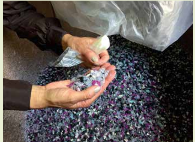
The Charleston East sustainability team toured local plastic recycling facilities to find a home for various plastic waste streams generated during construction. HDPE plastic products, such as conduit and underground plumbing, are melted down and reformed into new products.
