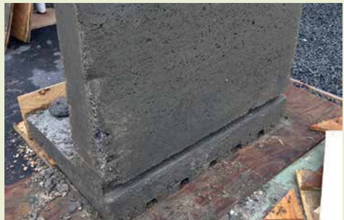
As proof of concept, the designers made a 1:1 mock-up of the fluted concrete fascia to discuss buildability with the general contractor.
