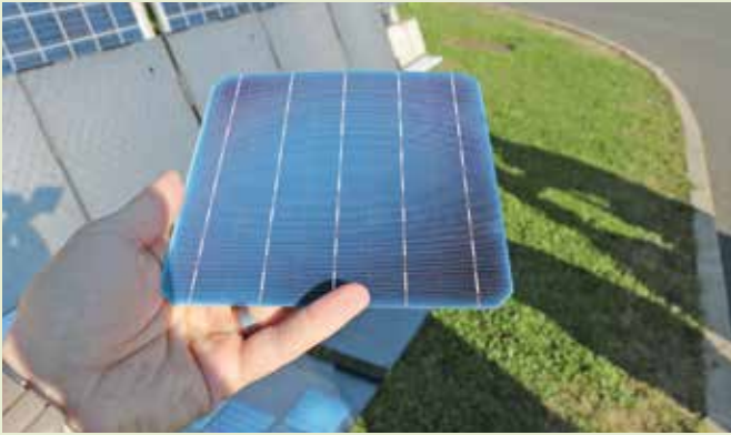
The team reviewed various color grades of photovoltaic cells and specified a tight range of color for use in the dragonscale shingles.
