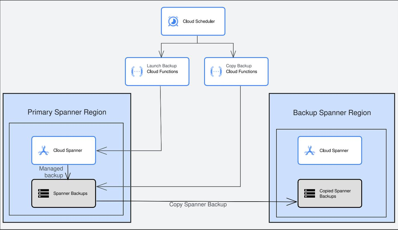
In the case of a failure scenario where the main region becomes unavailable, these backups in the backup region can be used to restore and populate a Spanner database in the backup region.
